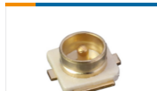
TE Part #CONMHF1-SMD-G-T U.FL/MHF1 Jack 50 Ohm PCB Surface Mount
