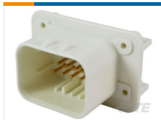
TE Part #1-776266-2 14POS,PIN DIA 1.3,HDR ASSY,90DEG, COD 2
