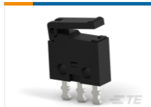
TE Part #2351460-1 MINSA SW HLV 0.30N 0.5A AC SC UnPtch
