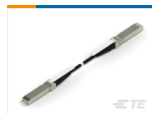
TE Part # CAT-C11-H5 SFP+ to SFP+ I/O Cable Assembly: 24 AWG
