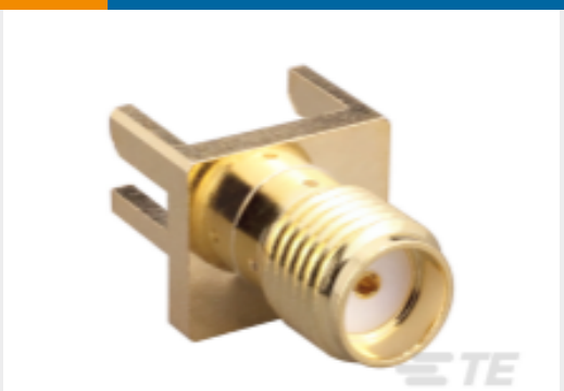
TE Part #L9000279-01 SMA Jack 50 Ohm .062 PCB Edge Mount
