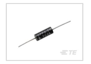
Resistor Type: Precision Resistor Passive Component Dimensions: 10.2 x 4 mm Number of Terminations: 2 Packaging Method: Bulk Passive Component Tolerance: .1 %
