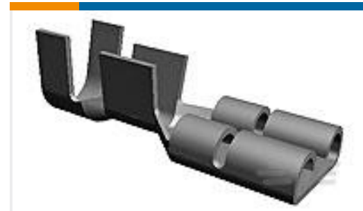
TE Part #63475-2 187 FASTON REC 20-16 AWG TPBR
