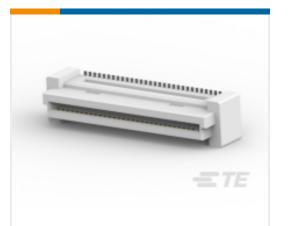
TE Part # CAT-313-RCB60 Free Height Receptacle Conn: Board-Board, Vertical, 60, 0.8mm
