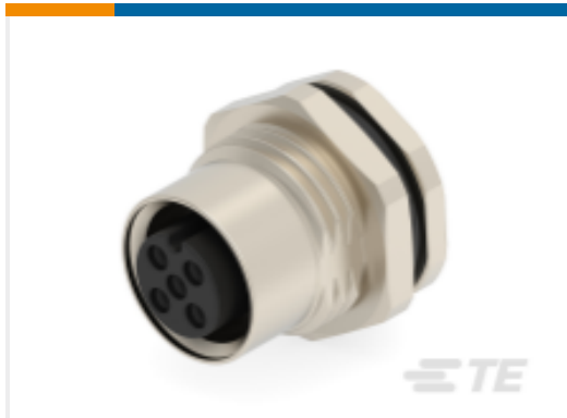
TE Part #T4131012021-000 M12,REAR MOUNT,FEMALE,A,2P, SOLDER WIRE
