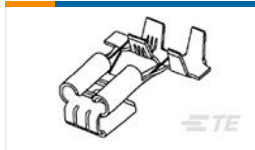
TE Part #151321-4 250 FASTON,FLAG,REC.,18-14 AWG, TPBR
