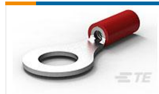
TE Part #342105-1 TERM, RT, PLASTI-GRIP, 22-16, M6(1/4)
