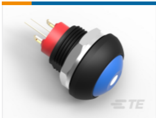
TE Part #2-2329387-1 PB OFF/ON FC BLU M1 TERM WHI LED IP68
