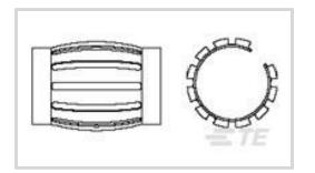
Contact Type: **Pin** Number of Positions: **1** Sealable: **No** Contact Current Rating (Max): **65 A** Circuit Application: **Power**
