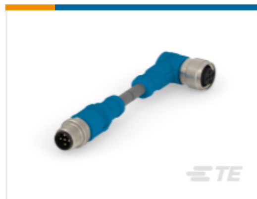
TE Part #T4162124005-001 RPC-M12-5MS-0.5SH-M12-5FR-PUR
