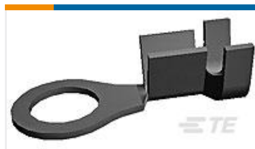
TE Part #160344-2 RING TONGUE 20-16 AWG .025 X .840
