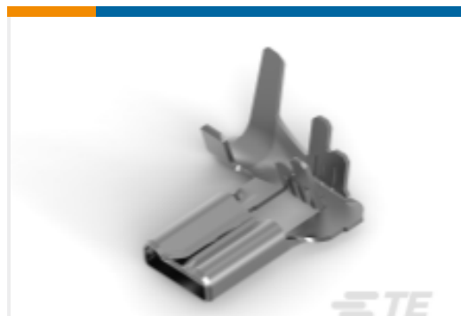
TE Part #2238172-3 187 FASTON,FLAG,REC.,24-14 AWG, TPBR
