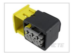
Connector System: Wire-to-Wire Number of Positions: 7 Connector & Housing Type: Housing for Female Terminals Centerline (Pitch): 4 mm, 6 mm [.157 in, .236 in ] Sealable: Yes
