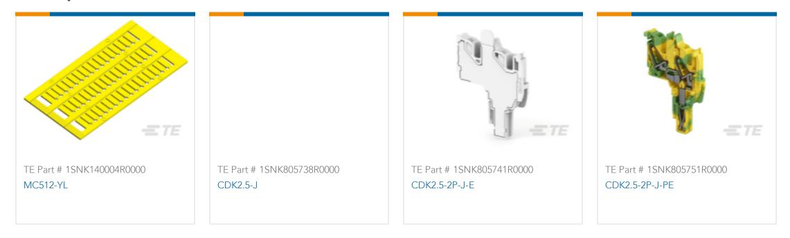
Modular Terminal Blocks, Feed-Through & Ground, Screw Clamp Terminal Block, Green & Yellow, Product Spacing .204 in [5.2 mm], 4 Position, ENTRELEC SNK
