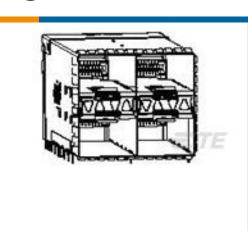
TE Part #2198325-6 zSFP+ STACKED 2X2 RECEPTACLE ASSEMBLY
