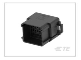
Connector Product Type: Housing Connector & Housing Type: Housing for Male Terminals Connector System: Wire-to-Wire Number of Positions: 32 Centerline (Pitch): 2 mm [.079 in ]
