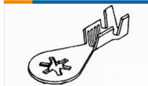
TE Part #61795-3 RING 18-14 AWG TPBR
