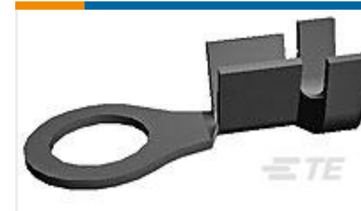
TE Part #160344-2 RING TONGUE 20-16 AWG .025 X .840
