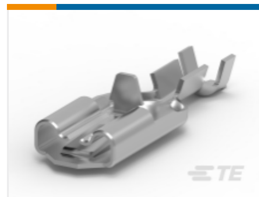
TE Part # 2238156-1 POS LOCK 250 Rec, MKII, 22-18 TPBR
