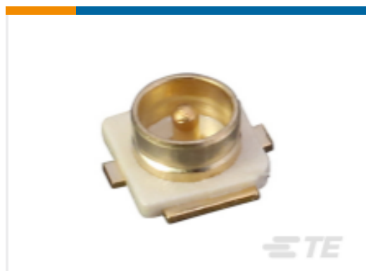
TE Part #CONMHF1-SMD-G-T U.FL/MHF1 Jack 50 Ohm PCB Surface Mount
