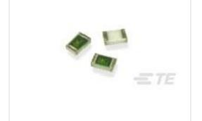
TE Part #1676246-2 RN 0805 1K96 0.1% 10PPM 1KRL
