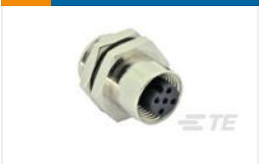
TE Part #1838891-2 M12 Mtl FEMALE PNL CONN. Sldr Rear (Hex)
