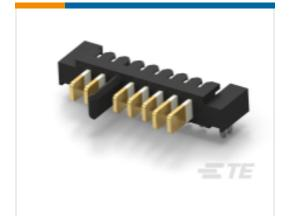
TE Part # 1827654-1 2mm pitch Battery Plug Assy. 7Pos. H=4.0
