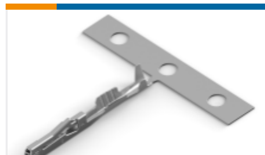
TE Part #2834464-6 MD REC CONT TIN 22/24 AWG
