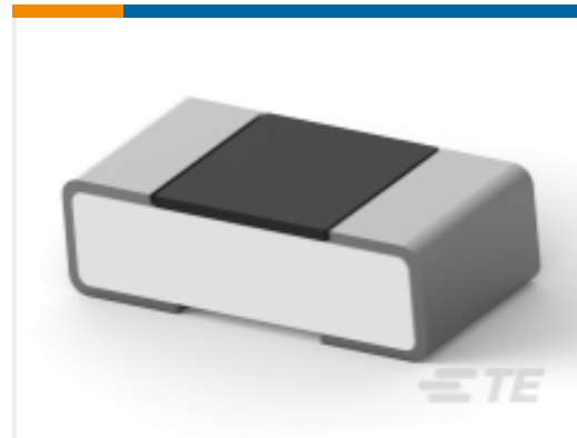
TE Part #4-2176363-1 RQ 0402 1K13 0.1% 10PPM 5K RL
