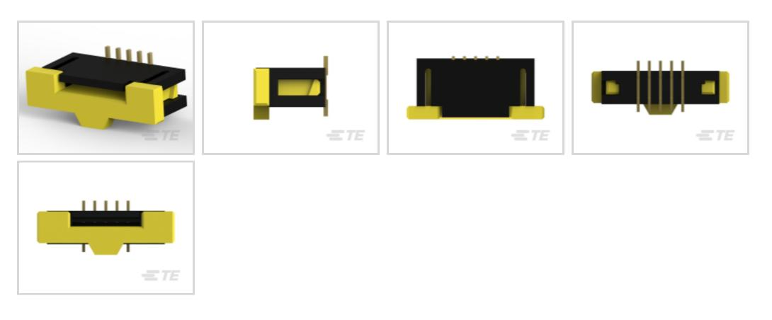
Connector System: Flex-to-Board Number of Positions: 5 Centerline (Pitch): 1 mm [.039 in ] Insertion Force Type: Zero Insertion Force (ZIF) PCB Mount Orientation: Vertical
