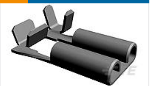
TE Part #1742087-2 187 FASTON, FLAG, REC., 18-22 AWG, TPBR
