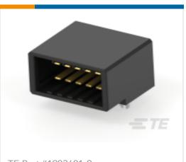
TE Part #1903601-2 Header Assembly: Wire-to-Board, 15A, gold or tin plated
