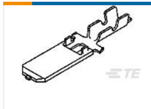
TE Part #170341-3 FF 250 TAB 14-12AWG PTBR WITHOUT LATCH
