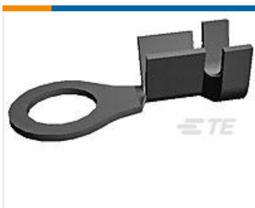
TE Part #61844-1 RING TERMINAL 12-10 AWG .0395X.650 TPCU
