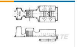
TE Part #160739-4 250 FASTON,PIGGYBACK REC.,18-14 AWG,TPPB
