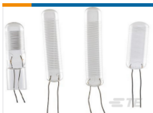
TE Part #32205074 GX518 1Pt100 W0.15 L5/D1.8mm
