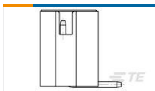
TE Part #1775470-6 HPI CONN., 2.0MM, V/T, SMT, 6P, 80U"
