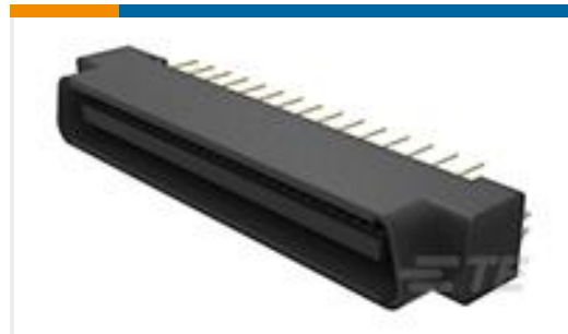
TE Part #1734100-6 Champ050 series,60pos,Au over PdNi
