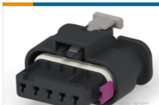
TE Part #1-2355515-5 5POS, MCON 1.2, REC HSG ASSY, SLD, COD A
