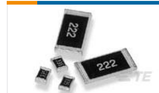
TE Part #3-1879502-2 CRGH2512 5% 270K 2W
