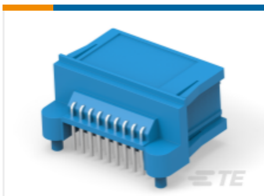
TE Part #6-1379731-3 18pos MQS .63 header 90deg THR
