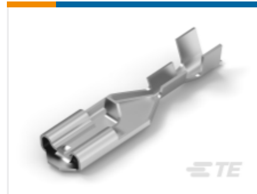
TE Part # 170324-6 POSITIVE LOCK 187 REC 24-20AWG 0.3 PTPBR
