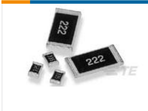
TE Part #1623402-1 CRG1206 1% 100K
