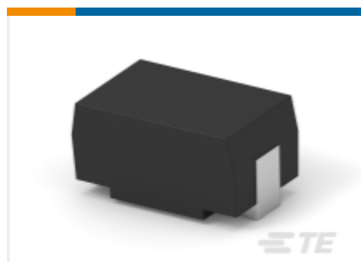
TE Part #5-1676966-3 SMD Power Resistor: 7 Watt, 200-2M Ohm
