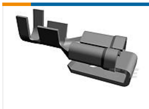
TE Part #62026-1 187 FASTON REC 20-16 AWG TPBR
