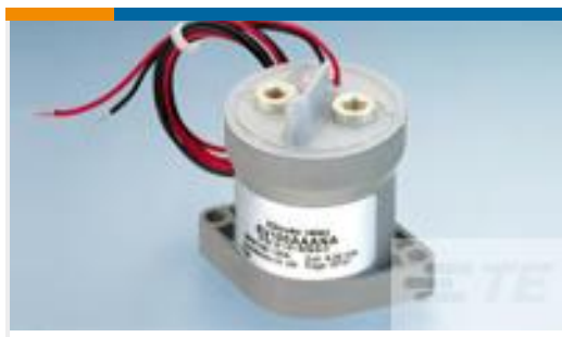
TE Part #5-1618398-0 EV100AAAANA=CONTACTOR, SPST- NO 9-36Vdc
