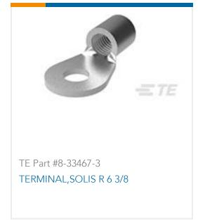
Closed Ring Tongue Terminal, 6 AWG, 3/8 Stud Size, 9.91 mm [.39 in] Stud Diameter, Closed Barrel, Straight, Tin, Uninsulated
