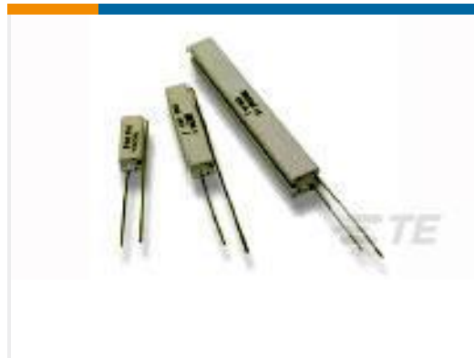
TE Part #1623729-8 BCHE 17 W 1K5 5%
