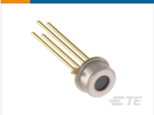
TE Part #G-TPCO-032 Analog Thermopile TO-18, FOV 110, NTC Ref
