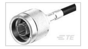
RF Interface: **N Type** RF Connector Style: **Plug** RF Connector Mated Outer Diameter (Approximate): **21 mm [.827 in ]** Impedance: **50 Ω** Compatible With RF Cable Type: **RG 393**
